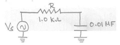
26. Determine the power factor, the true power, the reactive power and the apparent power in the circuit in fig.
