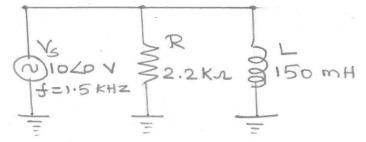
22. a) Convert the series parallel circuit in the below figure.to an equivalent parallel form at the given frequency.
