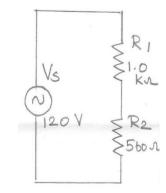
20. a) Determine the total admittance (Y)and then convert it to total impedance(Z) in figure. Draw the admittance phasor diagram.
