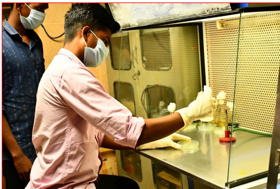
Fig. 23. Laminar Air Flow Chamber
