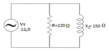
**10 a)** Find the current and the voltages across each component and draw a complex voltage phasor diagram.
